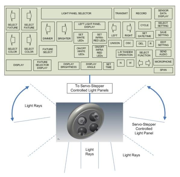
\*The Control Panel is designed specifically for your configured application and your specific light unit, which may have a different number of light panels. Specifications and features may vary from the description above. The features shown in the controller above are only a sample of over 122 available features. The Control Panels are designed to work with your specific version of Uriel Corporation's S.A.L.T.<sup>™</sup> LED Lighting Systems.
